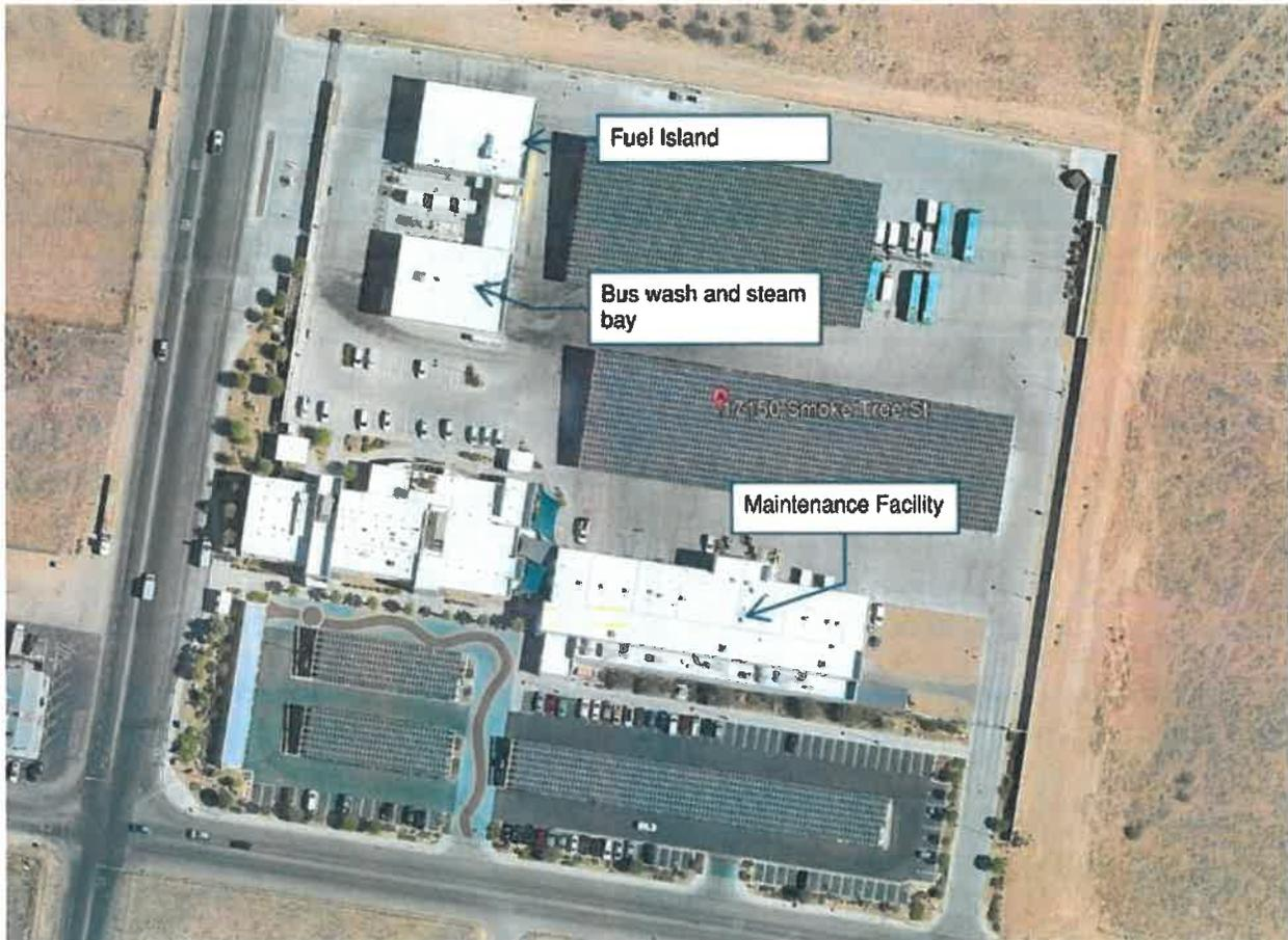
VVTA currently maintains and operates a fleet of compressed natural gas (CNG) buses. Currently, the facilities are equipped to work on and fuel CNG buses. VVTA is in contract to add a Hydrogen Fueling Station with two (2) H2 dispensers being placed at VVTA's current fuel island located on the north-west side of the facility.
